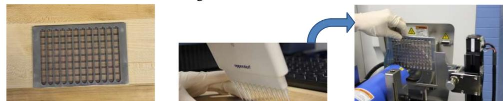
FIGURE 1. – Screen holder assembly with steel mesh. A 12-tip pipette spotting milk samples. The assembly being lowered into the XZ transmission module
