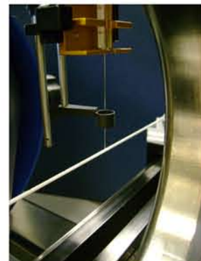
Figure 10. Liquid sample handling with CTC PAL syringe and direct spotting onto ceramic rod.
