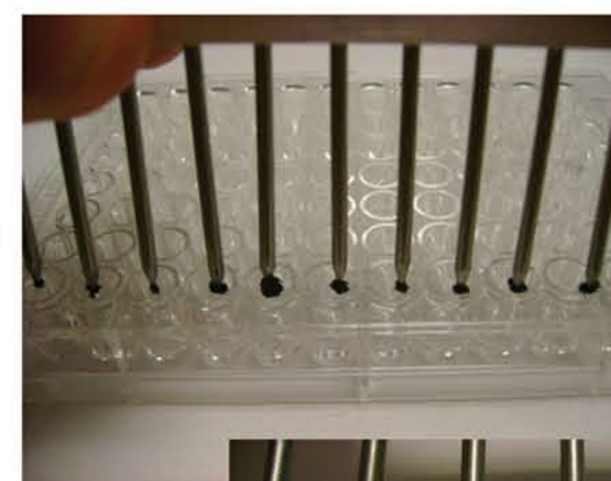
Figure 3. Powder analyte mixed with magnetite (2 mg total mixture weight) were placed into the wells of a 96-well microtiter plate. A custom piece with extended ferromagnetic pins spaced to correspond with one row of a 96-well plate was topped with a strong (3080 Gauss) neodymium bar magnet. The block was dipped into the sample wells, collecting all the powder.
