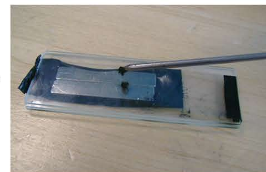
Figure 2. Metal powder is transferred to the glass slide with a magnetic micropipette and held in place by the neodymium magnet underneath.
