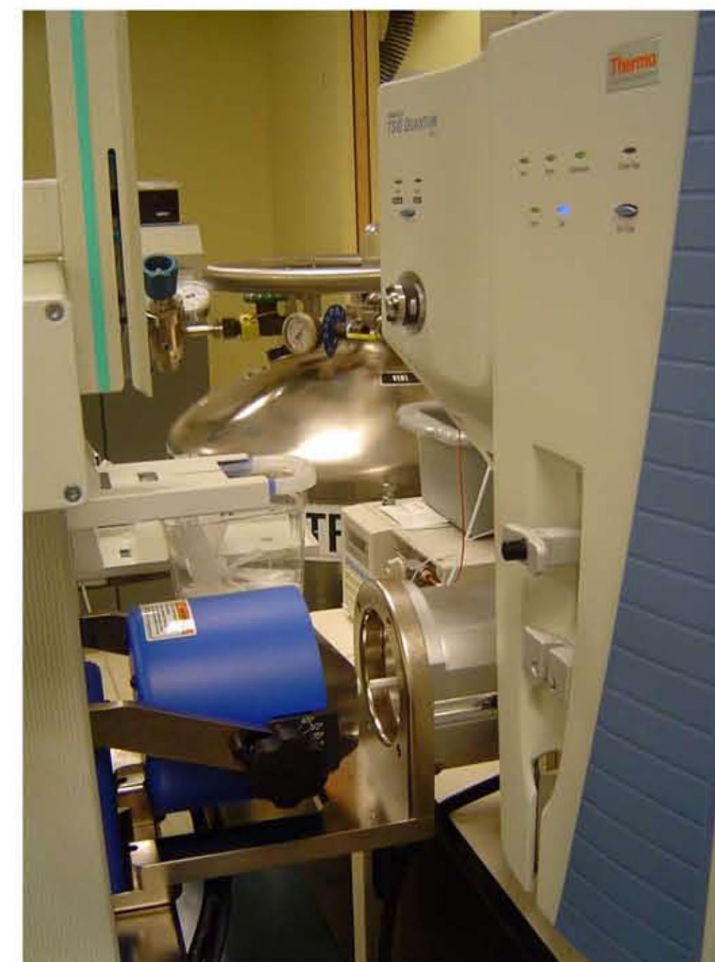
Figure 1. DART-ET ionization source mounted with a Vapur Interface on a Thermo Quantum Ultra triple quad MS.
