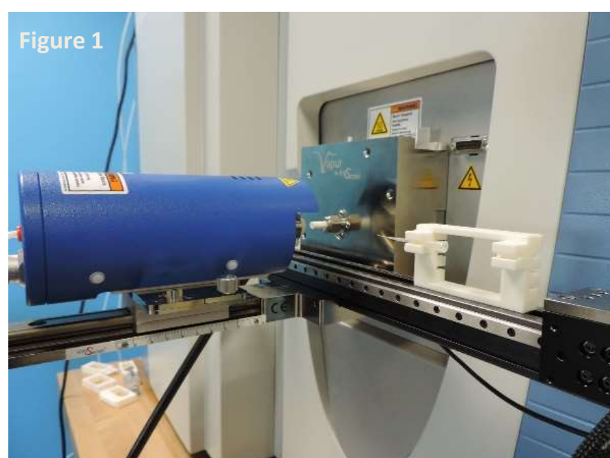
FIGURE 3. Multiplex SPME sampling apparatus. Allows for simultaneous sampling of multiple SPME fibers
