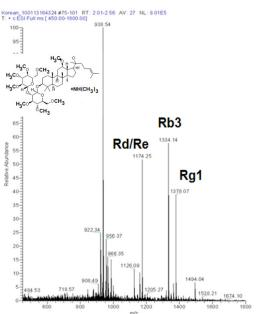
Detection of the intact ginsenosides and the major fragment at 938 dalton from loss of the disaccharide provide a mass spectrum that characterizes the root.
