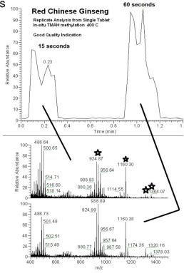
Sample preparation is minimal. The DART driven reaction occurs rapidly. In a non-automated configuration sample analysis is complete in less than 1 minute
