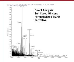
Possibilities for process monitoring are evident with the rapid detection of changes in ginsenoside distribution after sun drying, a common practice in production of traditional medicines (above)
